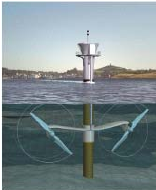
Figure 3. Marine Current Turbine's SeaGen dual-rotor turbine
